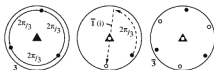
Fig. 8.9. Regular three-fold rotation axis, operation of a three-fold roto-inversion and result of the repeated operation of the roto-inversion \bar{3} .
