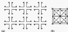
Fig. 10.5. (a) Kockel diagram of a symmetric 2-D structure and (b) its unit mesh and symmetry operations.
