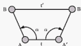
Fig. 8.4. Lattice translation vector, \mathbf{t} , connecting points A and A'. The lattice points B and B' are generated by a rotational symmetry axis (rotation by \alpha ) normal to the plane and passing through sites A or A', respectively.
